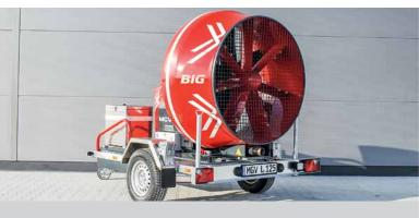
A purpose-built, special designed one-axle trailer. Compact and light-weight for extreme handiness. One person can easily position the MGV® with the big handles on both sides.
