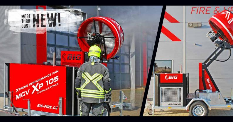
The Xtreme Performance fan XP105 and XP125 are the first hydraulically driven Mobile Grand Ventilators in lightweight construction. The newly developed large fans offer unique flexibility and extreme performance for the tactical ventilation of large-volume objects. The enormous inclination range of + 40 ° to -90 ° even enables vertical ventilation via openings at ground level, such as ventilation shafts and supply ducts. The patented lifting and tilting device allows a huge range of operations.
