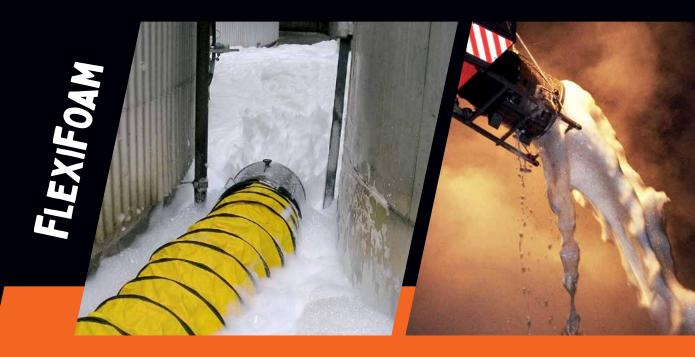
The FlexiFoam is connected to a high performance fan or a Mobile Grand Ventilator with ventilation hoses. The connection is made via a suitable duct reducer. In addition to the standard version, the gray ventilation hoses are temperature-resistant up to 180 °C and can be used close to the fire site due to the internal cooling by the fresh air. The water foam-agent mixture is supplied via a conventional hose line and existing premix systems.
